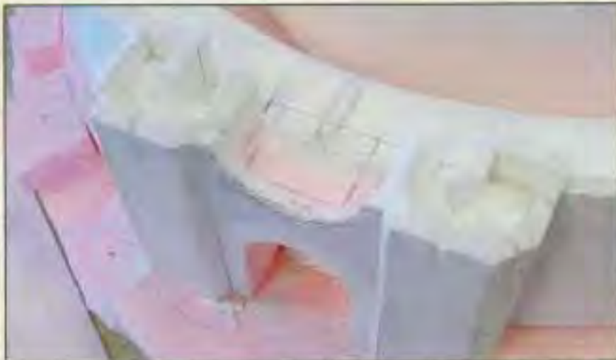
The edges of the battlements were thickened with foam and then carefully chamfered.
